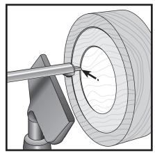
2. From the centre work the tool outwards to the required size.
