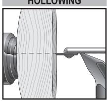
1. With tool rest on centre, place the flat face of the Multi-Tip tool on the rest. This gives more control and allows aggressive hollowing.
