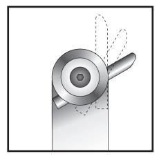
3. Angle of the cutter can be adjusted through 360°.
