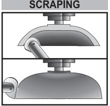
5. Fit scraper cutter using allen screw provided. Rotate cutter to required face - round faces for internal work, square face for external finishing.
