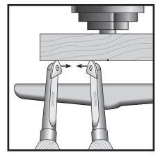
7. To create an even finer finish angle the tool at 45° on its curved back and work in either direction, this produces a slicing cut. Tool rest should be above centre.
