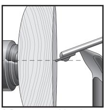
6. Place tool rest slightly above centre and with the flat surface of the tool on the rest trail the tool by approximately 5°.
